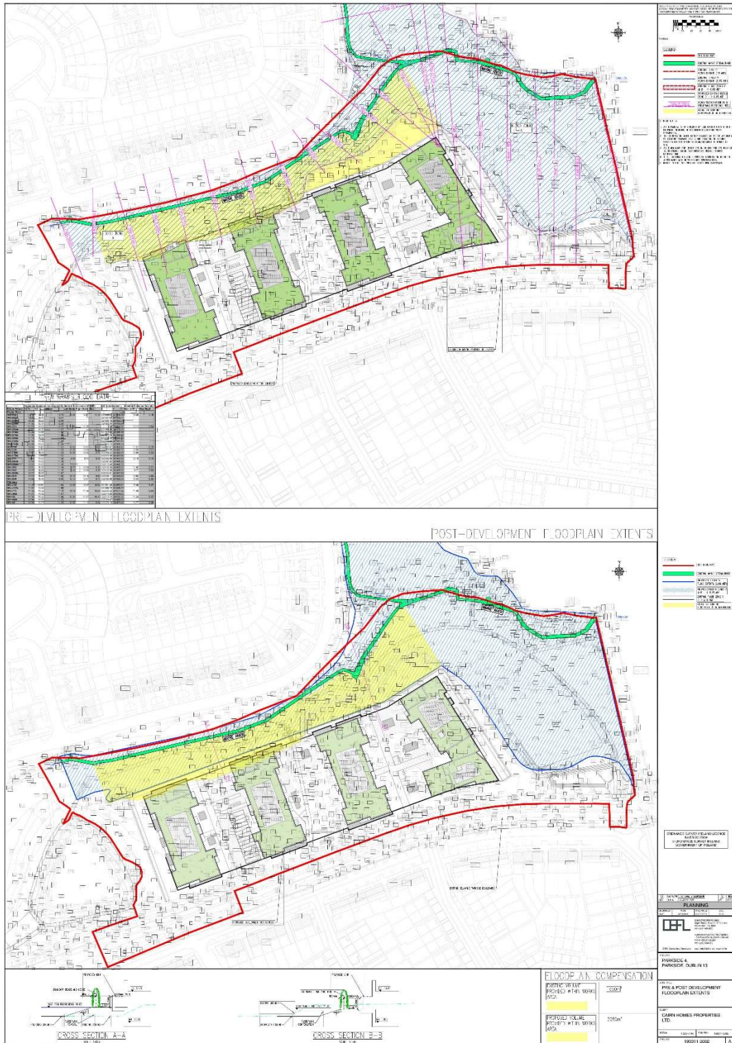
Figure 4 – Extract from the Flood Risk Assessment showing the existing flood zone (above) and the proposed changes (below).
